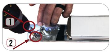
3. If your device has dogging, you need to **remove**TAIL PIECE BOTH SCREWS FROM CONNECTING ROD.
